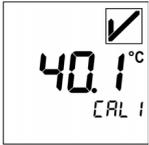
At the end of the "Measuring Time", the average value of the logged data will be calculated and displayed. Additionally, the indicator shows "pass" or "fail" according to the "Allowed Tolerance".
