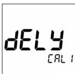
The calibration starts after pressing the TRANSIT-button. The data logger is waiting until the "Start Delay" time has elapsed.
