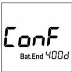
The configuration mode is used to define all logging parameters (profile). The liberoCONFIG is used to set or change all logging possibilities.
