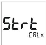
After the data logger has been configured, it is waiting for the start of the calibration.
