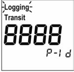
If "Show Profil-ID on LCD" is selected, the ID will be shown after the display test.
