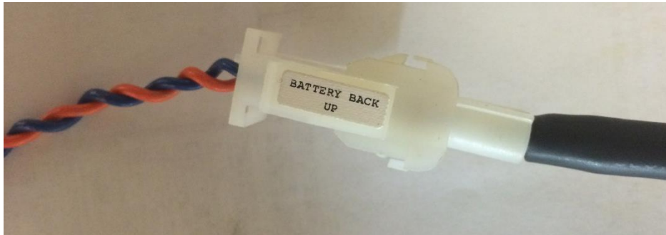
Battery Backup Connector. [Black – From the Battery Backup. Dark Blue/Orange – From the Chart MVE TS Wiring Harness]
