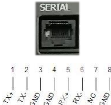
Figure 10: Chart MVE TS serial port and RS-485 4-wire pin diagram
