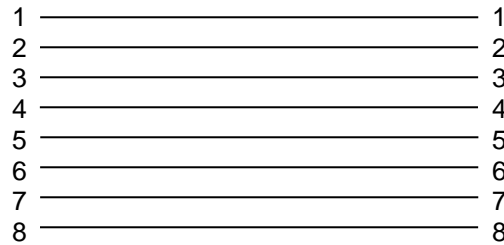
Figure 19: Standard reverse RJ-45 network cable configuration. Numbering as viewed from side of connector opposite latch.
