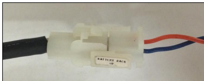
Battery Backup Connector. [Black – From the Battery Backup. Dark Blue/Orange – From the Chart MVE TS Wiring Harness]
